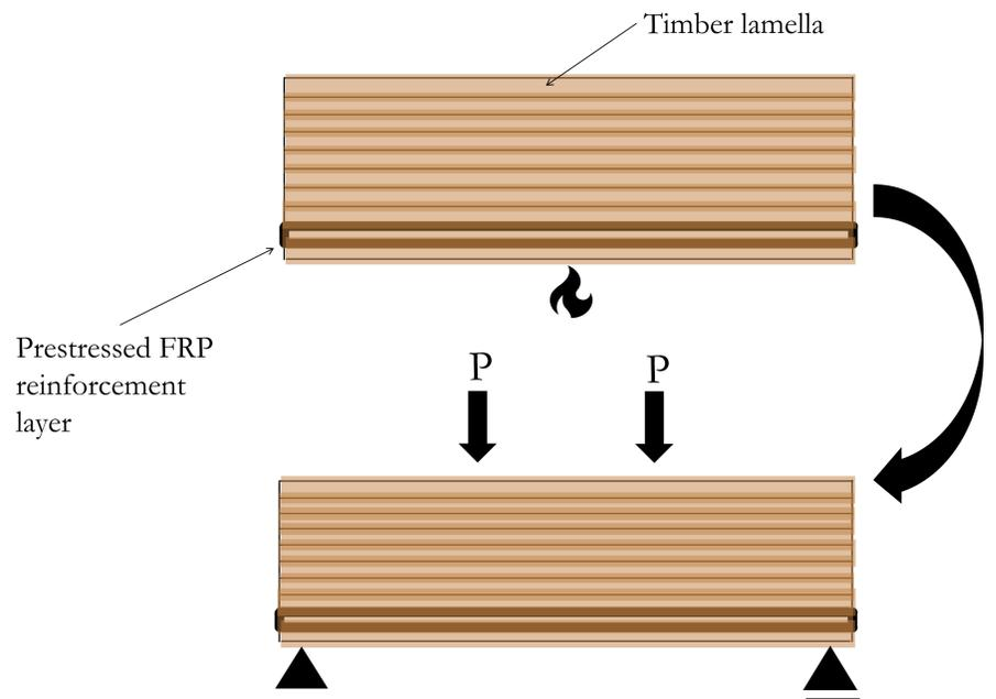
Residual testing of strength of composite material, in comparison with unreinforced beams to demonstrate the benefits of the FRP.
