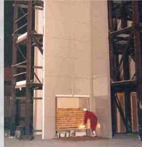
Figure 1. Natural-scale cladding test
