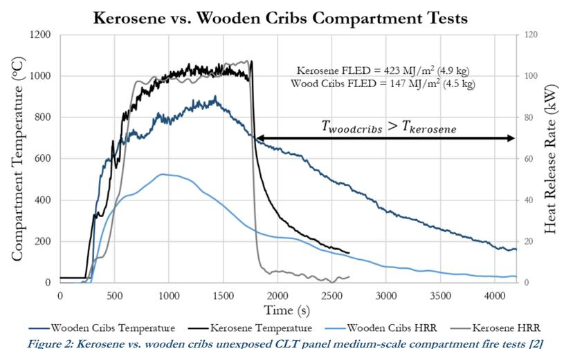
Figure 2: Kerosene vs. wooden cribs unexposed CLT panel medium-scale compartment fire tests [2]
