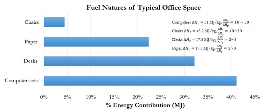
Figure 1: Contribution of specific materials to fuel loads with a typical office space with fuel load density of 220 MJ/m<sup>2</sup>
