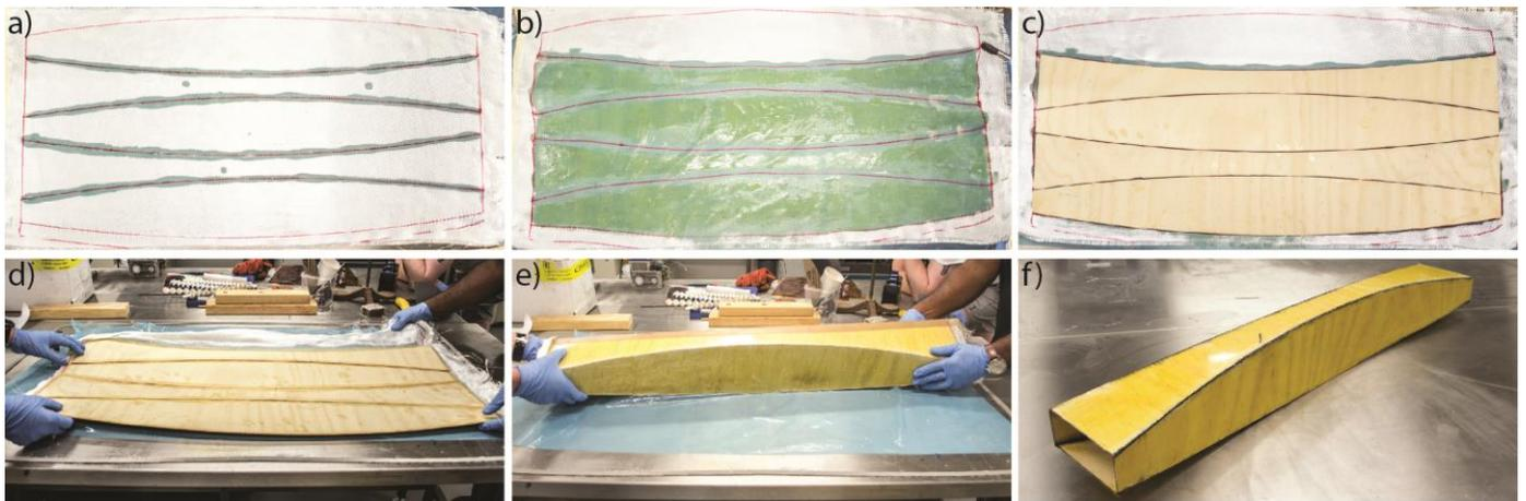
**Fig. 01** Innovative folded FRP-timber manufacturing process. a) Application of slow-cure resin to hinge regions. b) Application of fast-cure resin to panel regions. c) Application of thin plywood panels. d)-e) Folding following initial 3 hour cure. f) Final folded prototype.
